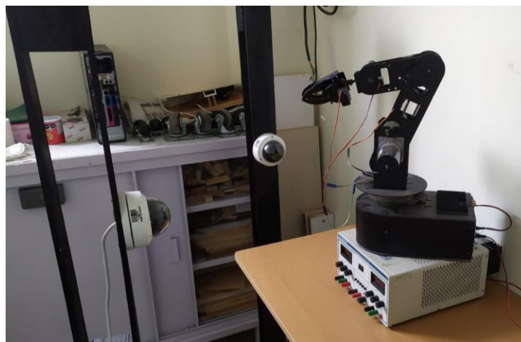
Figure 8. Preview of IP Cameras focusing on the robot arm.
